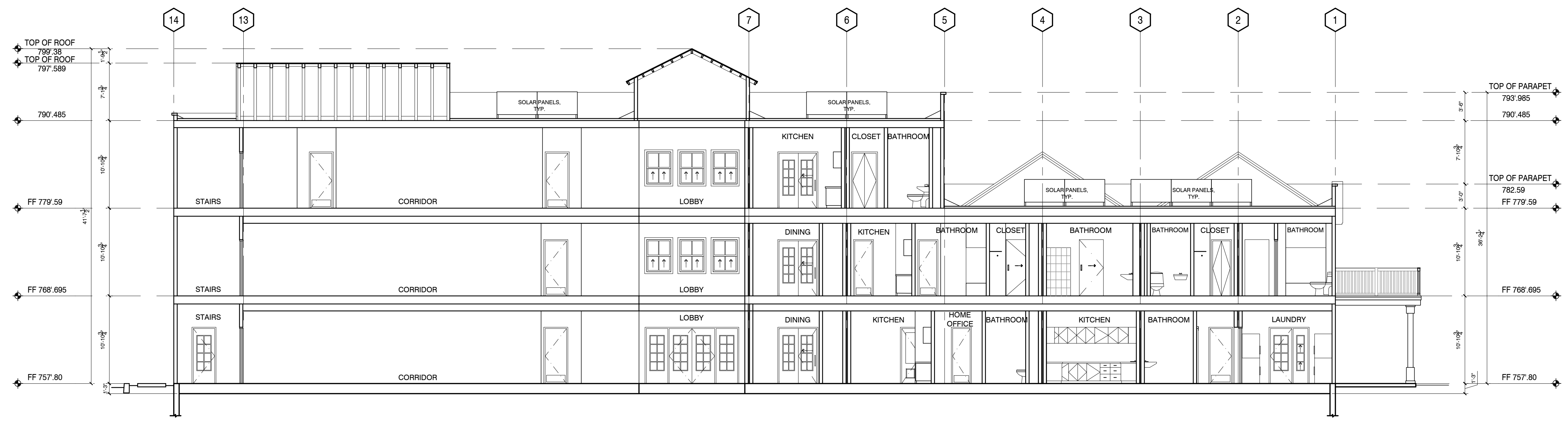
1 NORTH BUILDING SECTION SCALE: 1/8" = 1'-0"
